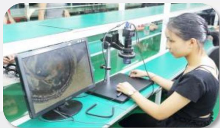
Solder joint inspection 焊点检测
