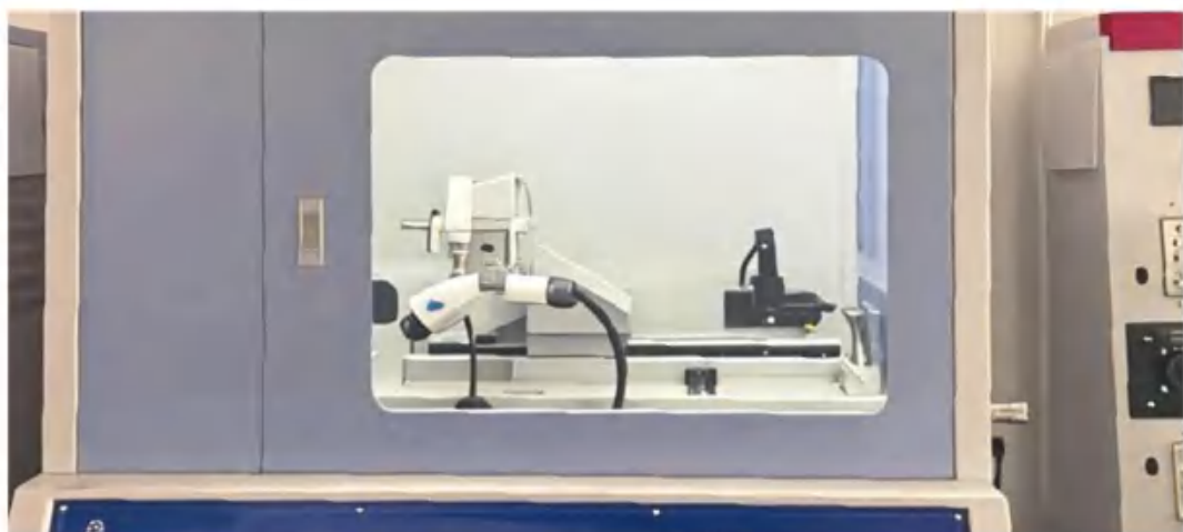
Plug-in/Press Tester Tests connector durability and mechanical lifespan
