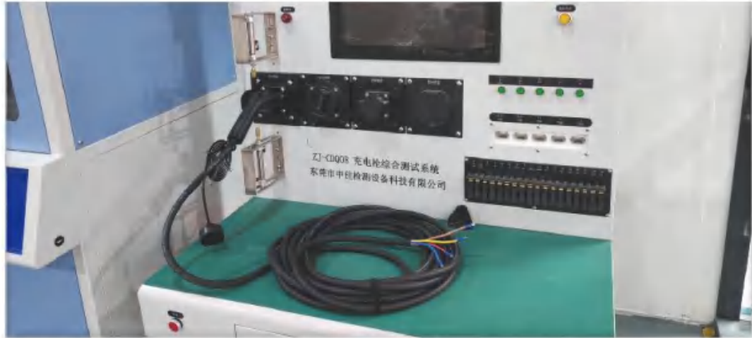
portable ev charger & Cable Tester Ensures safety and optimal performance of charging devices
