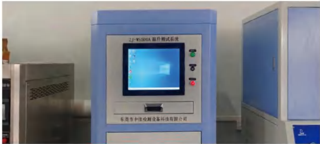
Environmental High & Low Temperature Tester Simulates extreme conditions to verify product stability
