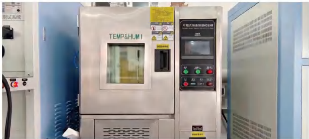
Component High & Low Temperature Tester Rigorously tests key parts for temperature tolerance
