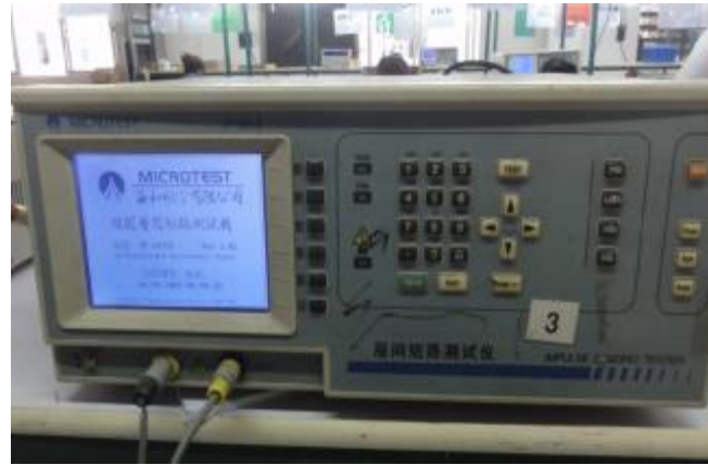
Layer insulation test
