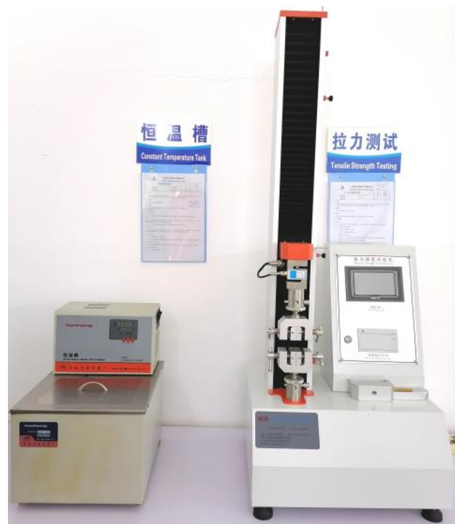
Constant Temperature Tank & Tensile Strength Testing
