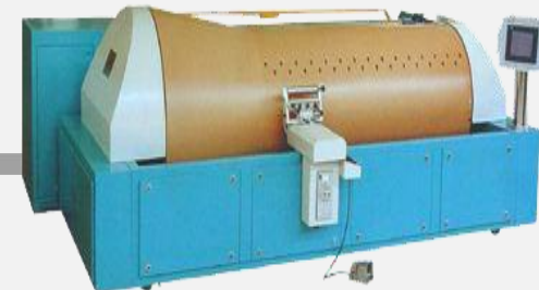
3 Beam Warper Machines
