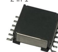
High-frequency isolation transformer
