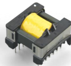
Main power transformer
