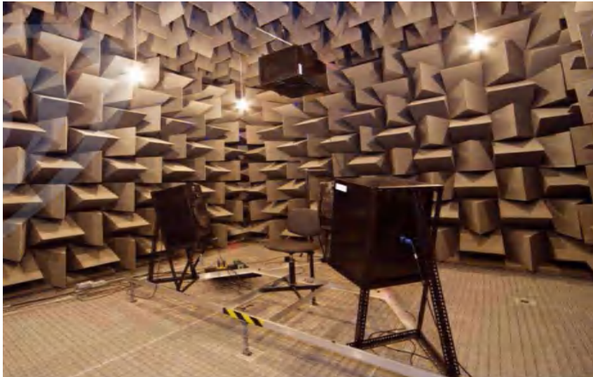
Anechoic chamber (11.5dB certification)
