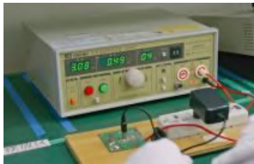
DC Electronic Load test
