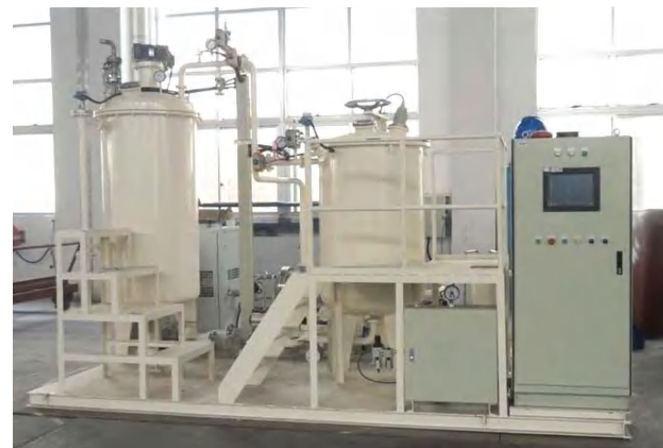
KI-600真空浸漆設備(特殊含浸) Special vacuum varnish machine
