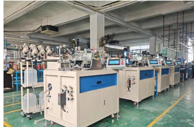
全自動多繞組單軸繞線包膠布 Fully automatic mutiple-windings taping and winding with single shaft
