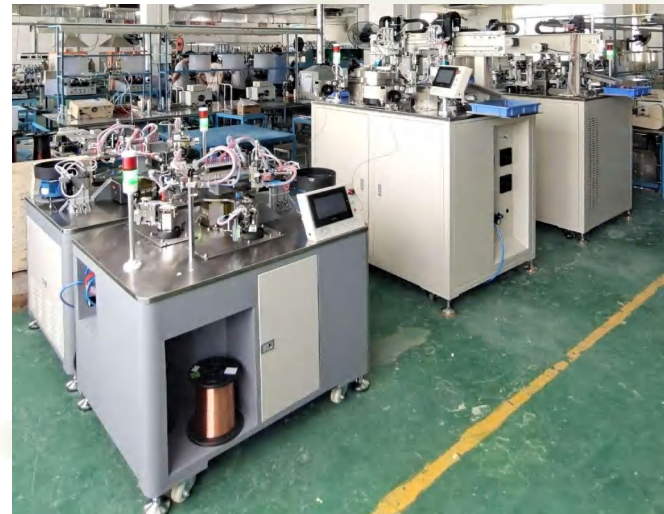
磁環全自動繞線 Fully automatic winding for toridal coils
