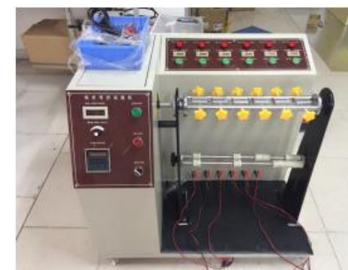
Wire bending test
