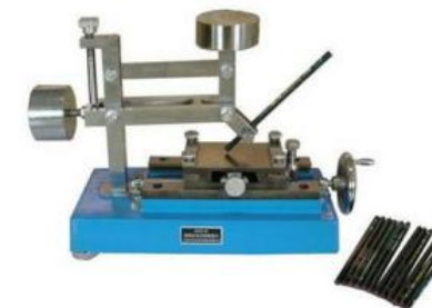
Pencil hardness test
