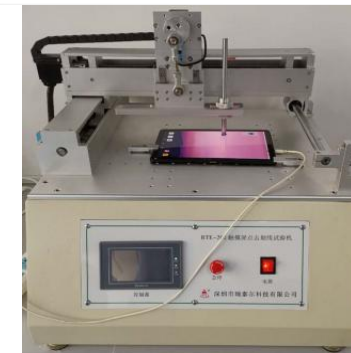
Touchscreen click and scratch test
