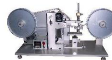
Touchscreen click and scratch test
