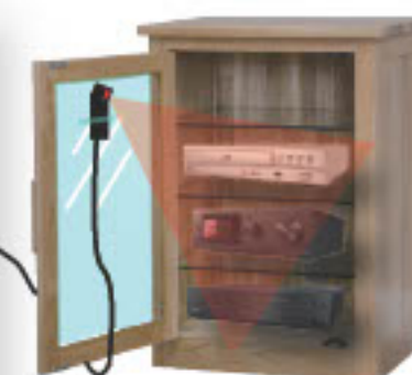
Cabinet with door installation: Attach emitter on door, roundshape facing the IR sensor.
