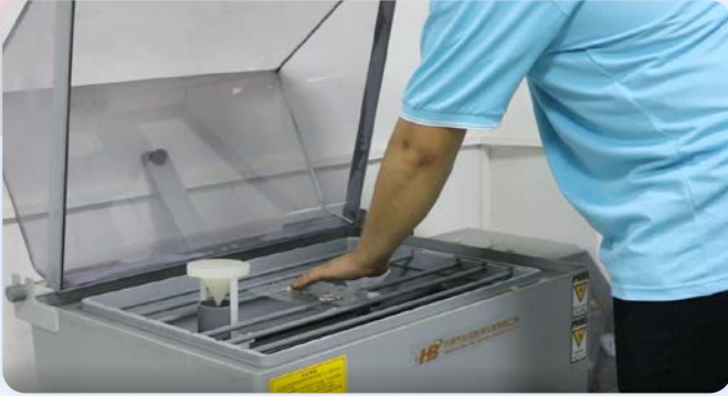
Salt spray test
