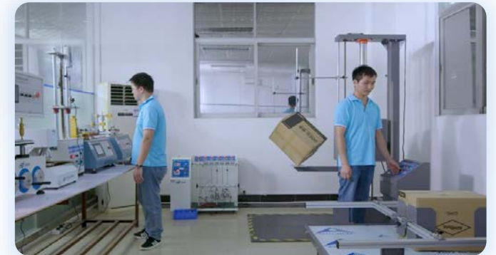
Transport swing and drop test
