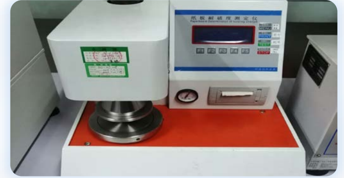
Paper board-Determination of bursting strength
