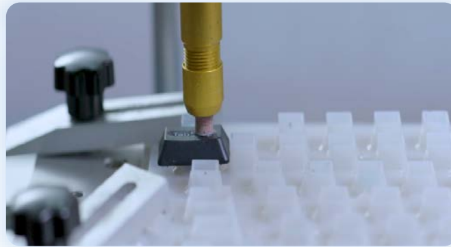
Wear resistance test
