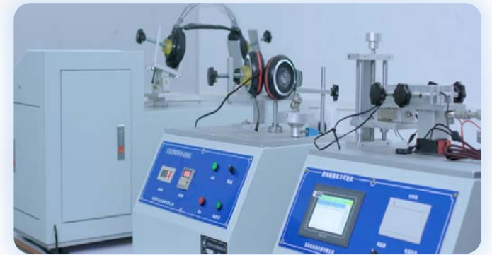
Quality test of headset headband
