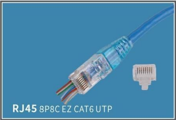
Designation:Cat 6 single-row EZ modular plug Conductor cavity OD:1.1mm Model Number: HX006UTK-W11 Applicable interface: RJ45
