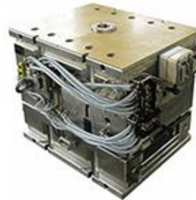
Hot runner injection mould
