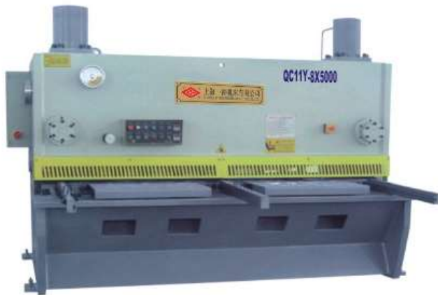
Hydraulic gate shears
