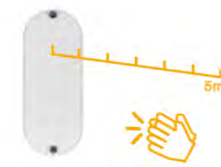
PIR sensor: 3-4m/25-30s/15-25lux
