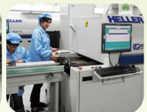
RoHS-compliant reflow machine
