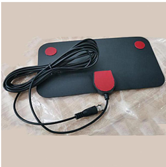
P/N:GLT001 Name:DVB-T Digital patch TV Antenna Freq: 174-240/470-862MHz Gain: 5dbi Dim: 210×120×0.8mm
