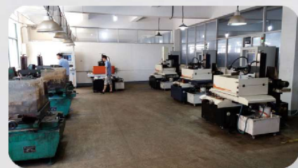
Wire-electrode cutting room
