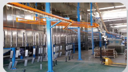
Automatic powder Coating Line
