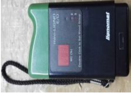
Humidity Test for the Timber
