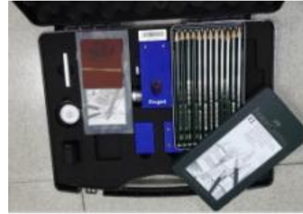
Hardness Test of the Painted Surface
