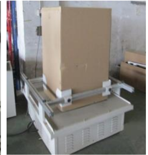
Vibration Test for the packaging
