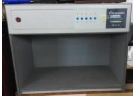
Specialized Lamp for checking the color
