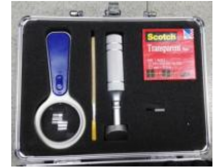
Hundred Cutter-Adhesive Force Test of painting
