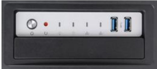
1*Power SW, 1*Reset, 1*Power LED, 1*HDD LED, 2*NIC LED, 2*USB3.0
