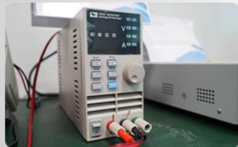
DC Voltage Regulator
