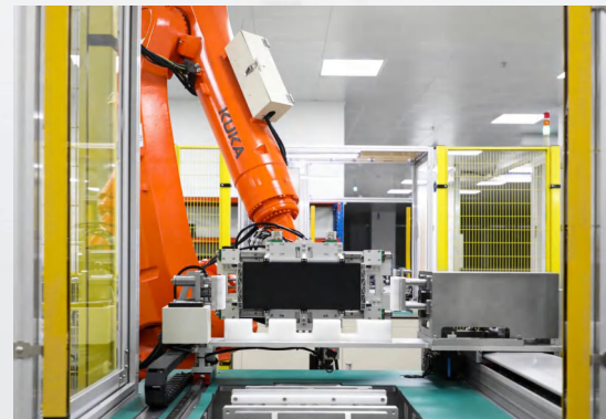
Fully automatic battery Pack module assembly line
