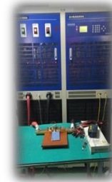
BTS-15V 800A Test Cabinet
