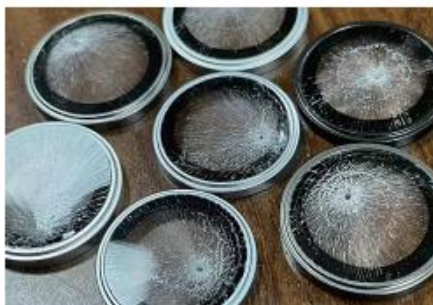
Individual camera glass with explosion-proof film, after the glass is broken.
