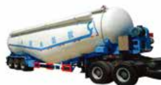
Cement Tank With Electrical Engine Drive
