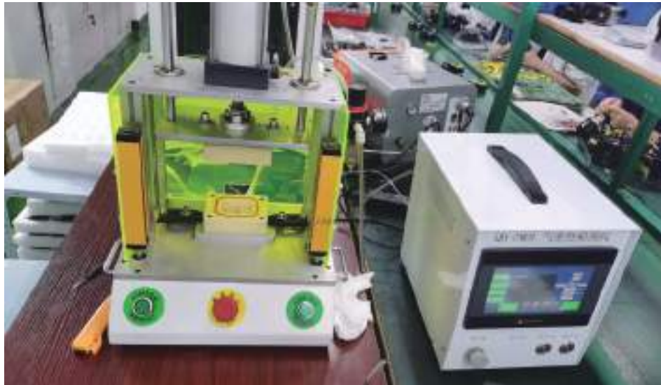
Air Tightness Tester (Waterproof test)
