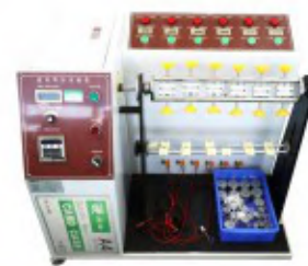
Wire Bending Testing Machine
