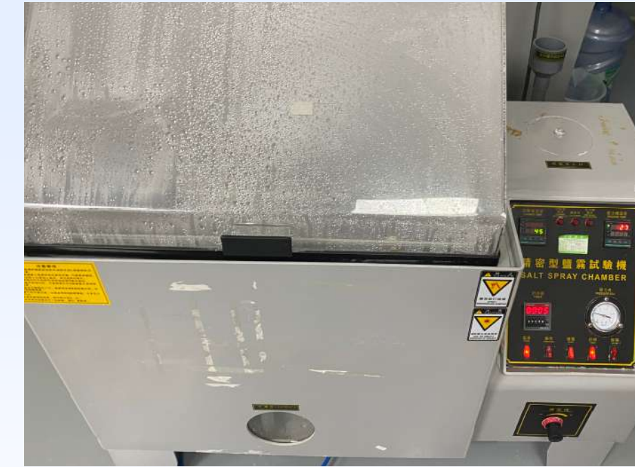
Salt spray test equipment Product corrosion test
