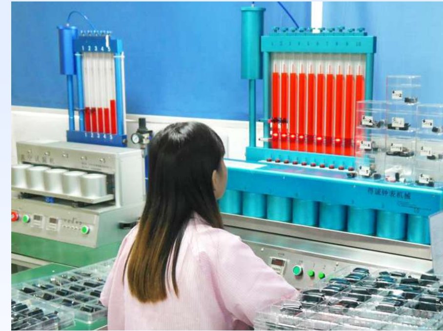
Semi-automatic air tightness testing equipment Detect product waterproof level
