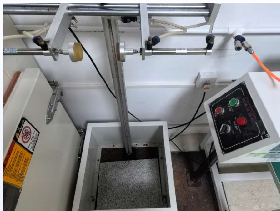
Drop test Verify the product's drop resistance
