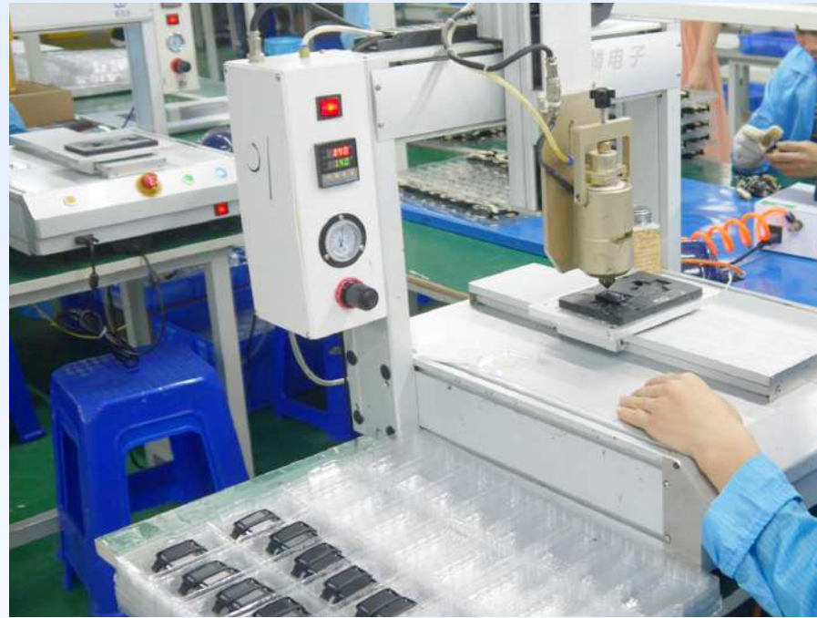
Semi-mechanized fast dispensing equipment Achieve waterproof effect
