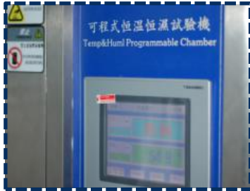
Constant temperature and humidity testing machine
