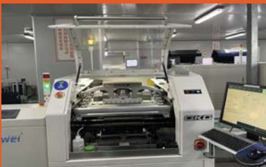
Automatic printing machine for solder paste
