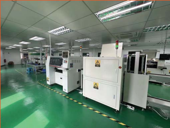
1 Automatic printing machine for solder paste
