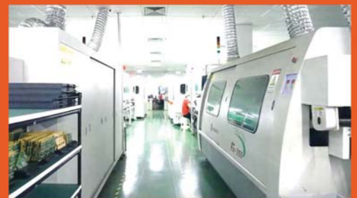
5 wave soldering line
