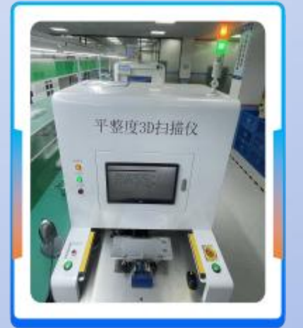
Infrared Flatness Detection
