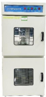
Battery explosion-proof experiment box
