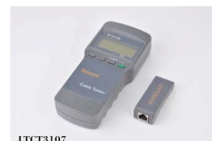
LTCT3107 Cable tester For UTP/STP RJ45 Cable, coaxial cable, telephone line. It is capable to have a number of tests such as cable connection, sequence, length, user jumper and cable connection continuity and determine any open circuit, short circuit, jumper or cross-talk interference.
