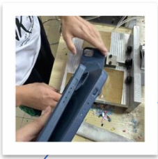
Bore the internal & external buttons Tear off the excess material
