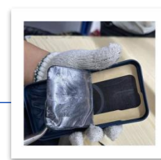
Tear off excess material
