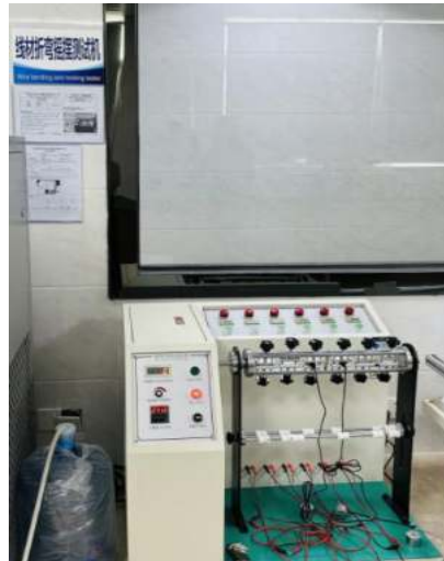
Wire bending tester
