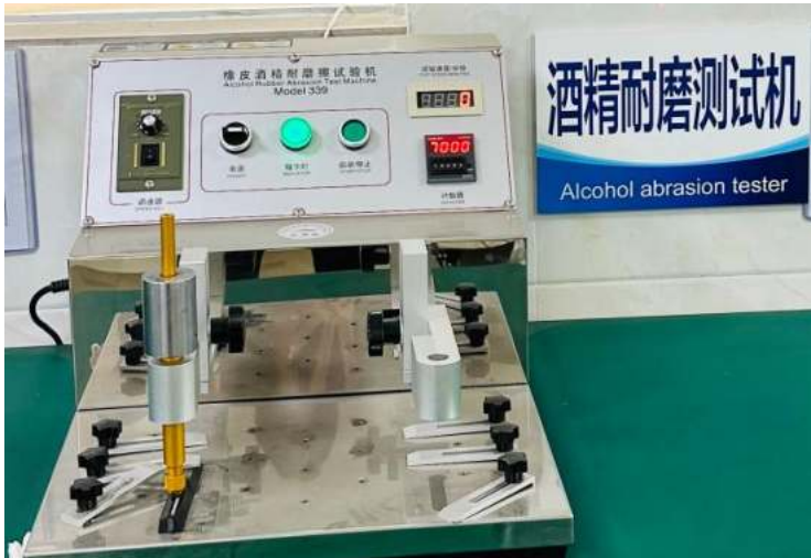
Alcohol abrasion tester
