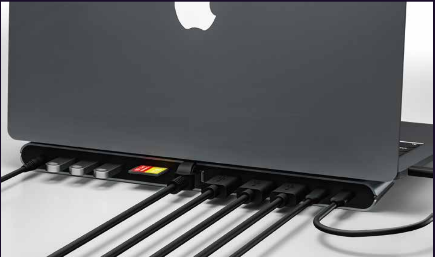
UC262 11 In 1 Type C Docking USB3.0*3+PD+HDMI*2+DP+RJ45+SD+TF+Audio
