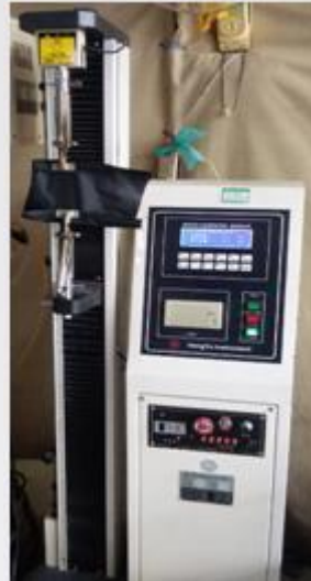
Fabric Strength Test
