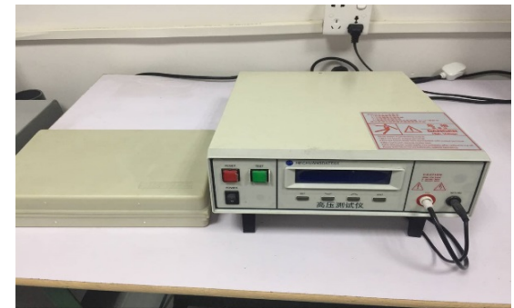
High Voltage Testing
