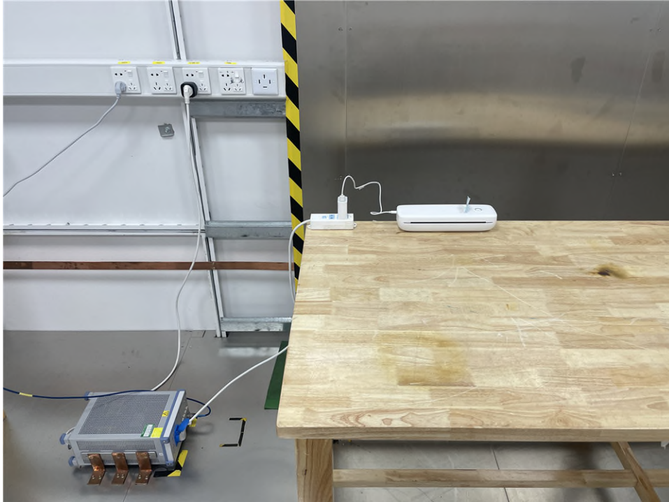
Photograph 1: Set-up for Radiated Emission (below 1GHz)
