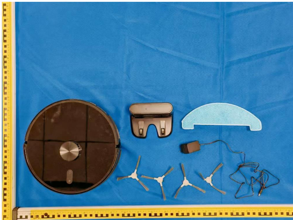
Figure 2: External view: EUT and detachable power supply unit (model: BZ019-190100-AG) + charging stand (model: V01)
