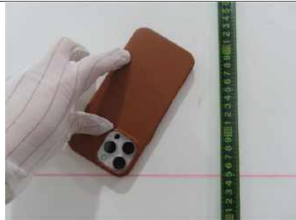
During test-Drop corner
