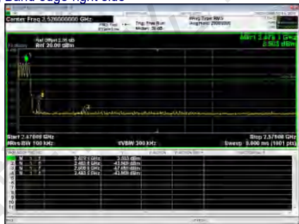
GFSK Hopping Band edge-right side
