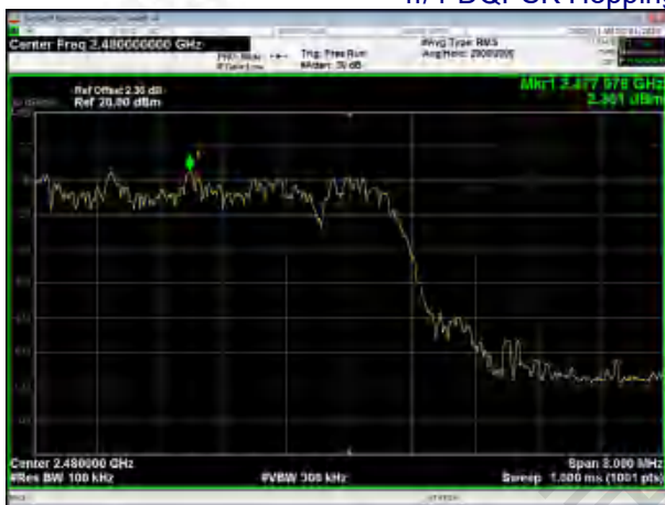
\pi/4 -DQPSK Hopping Band edge-right side
