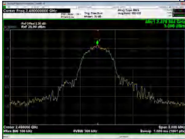
8-DPSK Hopping Band edge-right side
