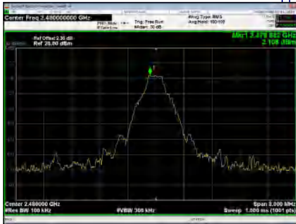
GFSK No-hopping Band edge-right side
