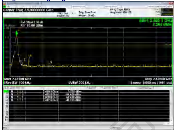
\pi/4 -DQPSK Hopping Band edge-right side
