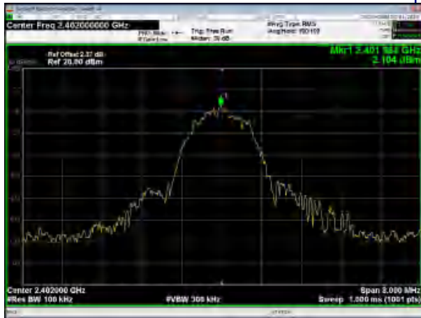
8-DPSK No-hopping Band edge-left side
