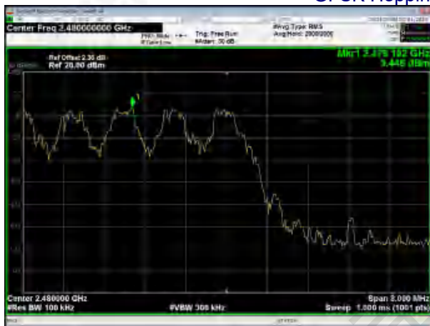
GFSK Hopping Band edge-right side
