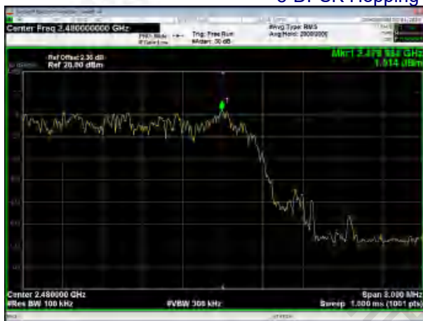
8-DPSK Hopping Band edge-right side
