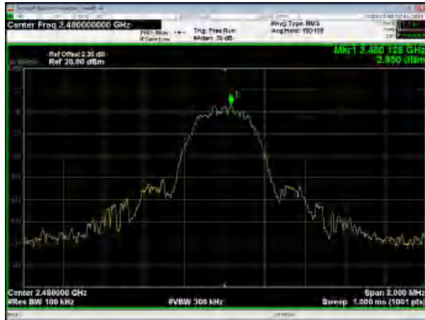
\pi/4 -DQPSK Hopping Band edge-right side
