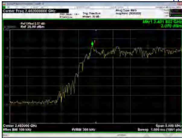
8-DPSK Hopping Band edge-left side
