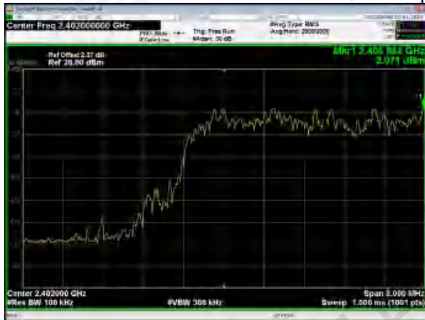
\pi/4 -DQPSK Hopping Band edge-left side
