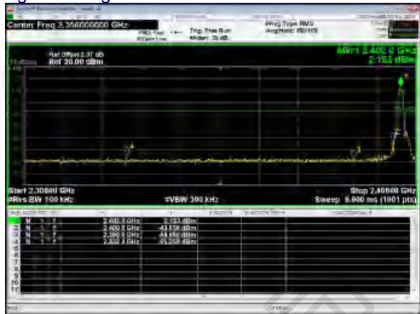
8-DPSK No-hopping Band edge-left side
