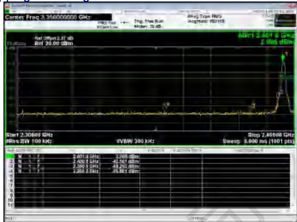
\pi/4 -DQPSK No-hopping Band edge-left side
