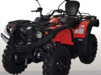
800cc ATV/tractor (HS234) • 4-stroke, liquid-cooled, twin V-type-cylinder, 8-valve EFI engine • 18.6KW (24.9hp)/4,200 rpm rated power;
