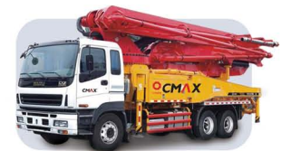
Truck-mounted concrete pump with 37m vertical reach and an Isuzu chassis
