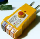
GFCI socket tester
