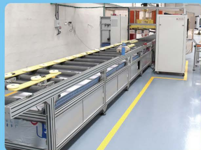
Automatic busbar inspection machine
