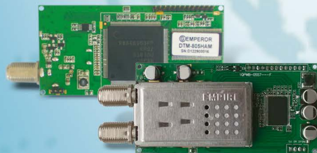
Digital TV tuner modules, ATSC/DVB-T/ISDB-T/DTMB/CMMB models available
