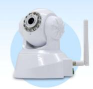
Plug-and-play IP camera with 1/4" CMOS sensor (N5402JV)
