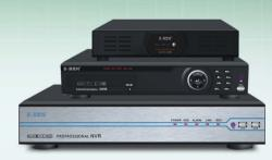
8-/16-/24-ch. NVRs (7B-N3000/6000/7000) 1080p recording
