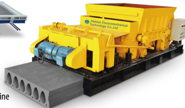
Automatic concrete slip forming machine
